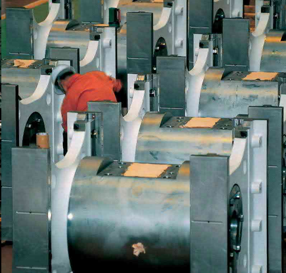
Crosshead pins with guide shoes.
