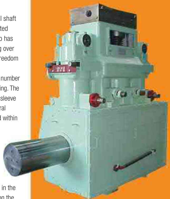
Pump housing with fuel injection pumps and exhaust-valve actuator pumps.
