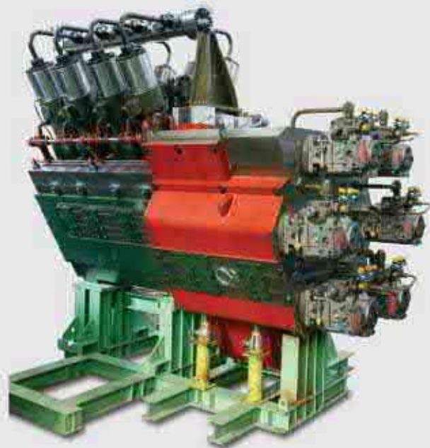
Supply unit for a 12RT-flex96C engine with the fuel pumps in Vee-form arrangement on the left and the servo pumps on the right of the central gear drive.
