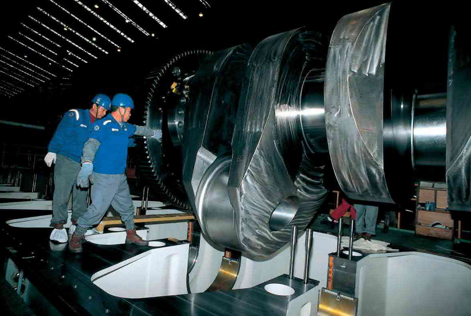
Lowering the crankshaft into the bedplate.
